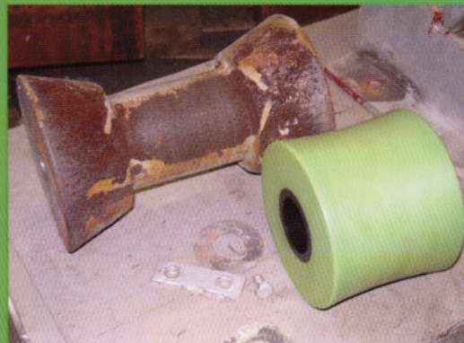
Petrobras – High Performance Plastic Rollers (RPAP®) installed on piers
